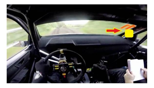
The GPS should be placed on the right pillar of the front part of the safety cage.
