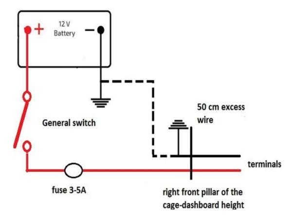
At the end of the cable there shall be fully insulated female blade-type terminals. 6.3X0.8mm
